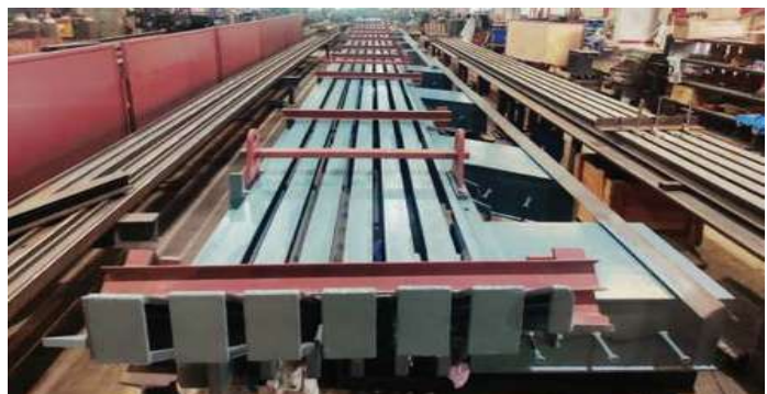
Swivel Joist Expansion Joints For Mumbai Trans Harbour Link (MTHL), Maharashtra
