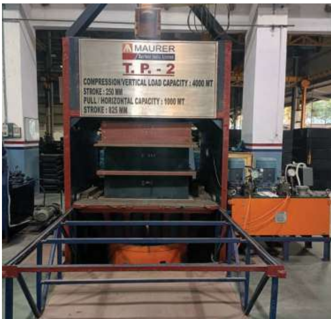
Testing of 2155MT Elastomeric Bearing
